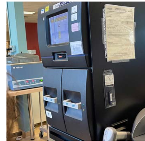
The bacT incubation machine, which tests for microbial contaminants in platelets that are intended for use in clinical settings.
